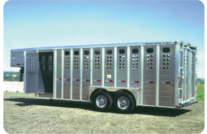
Merritt's punched aluminum panel construction keeps livestock well ventilated. The 34" wide driver-side swing door is standard on all Merritt Gooseneck trailers.
